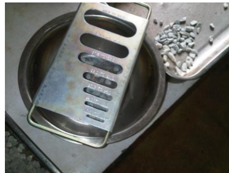
Fig. 15b Flakiness index gauge in action
