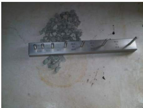
Fig. 15a Elongation gauge in action
